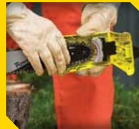
**ATTACH:** When the chain dulls from normal use, dirt contact, or rock strikes, simply attach the bar-mounted sharpener to the PowerSharp® guide bar. Twin guide holes in the tip of the bar make perfect alignment foolproof.
